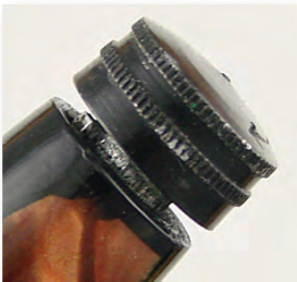
Fig. 8 Filler knob on twist filling fountain pen.
